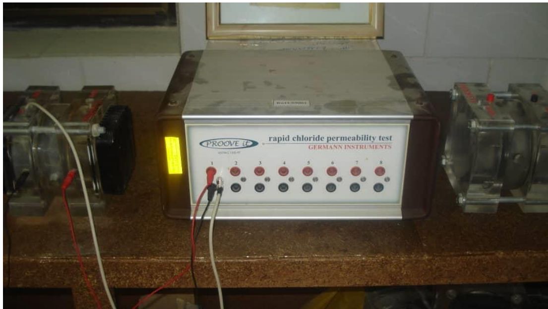
The device for determining the resistance to chlorine penetration by RCPT electrical conductivity method
